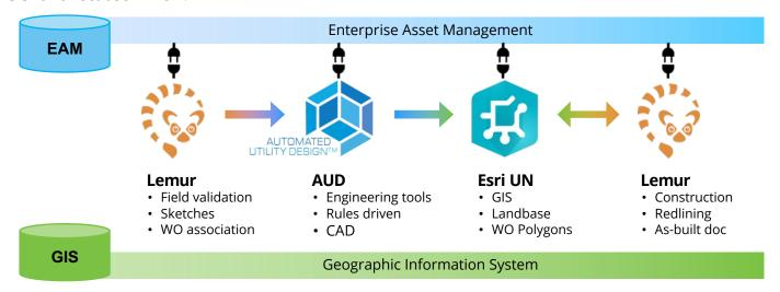
SBS's AUD is a CAD-based engineering design tool that works with GIS, creates GIS data, and validates the design as you build it. The user experience with AUD is seamless for designers trained on AutoCAD and gains the ERP benefits like automatic bill of materials creation. Designs built in AUD follow engineering standards, including rules from Esri's Utility Network.
